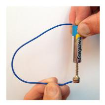
Magnets for "Spinning screws" (and "Invisible treacle") can be obtained from a variety of sources including Amazon. They are cylindrical magnets 10 or 12mm diameter. An AA battery works well and the wire can be stripped from any piece of cable. It does not matter if it is insulated or not, but if it is, then 1cm at each end should be bared.
