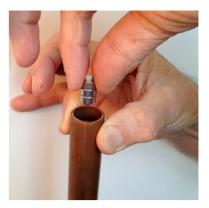
Magnets for "Invisible treacle" (and "Spinning screws") can be obtained from a variety of sources including Amazon. They are cylindrical magnets 10 or 12mm diameter.
