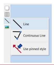
2. Click onto the document to set the start point for drawing the line, Drag across the page and Release the mouse button to set the end.
